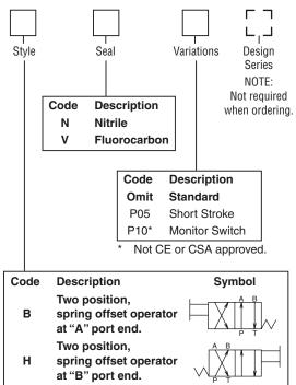
Valve schematic symbols are per NFPA/ ANSI standards, providing flow P to A when energized. Note flow paths reverse sides for #008 and #009 spools
