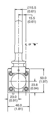
Note: 22.0 mm (0.87") from bottom of bolt hole counterbore to bottom of valve.
