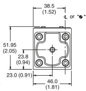
**Note:** 22.0 mm (0.87") from bottom of bolt hole counterbore to bottom of valve.
