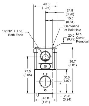
Note: 22.0 mm (0.87") from bottom of bolt hole counterbore to bottom of valve.
