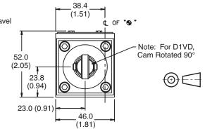
**Note:** 22.0 mm (0.87") from bottom of bolt hole counterbore to bottom of valve.
