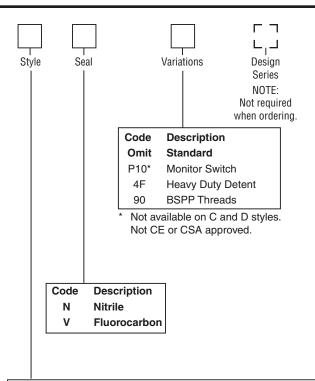
Code Description **Symbol** Single operator, two position B# spring offset. P to A and B to T in offset position. Double operator, С three position, spring centered. D Double operator, two position, detent. Two position, spring centered. E# P to B and A to T in shifted position. Single operator, two position, H# spring offset. P to B and A to T in offset position. Two position, spring centered. K# P to A and B to T in shifted position.
